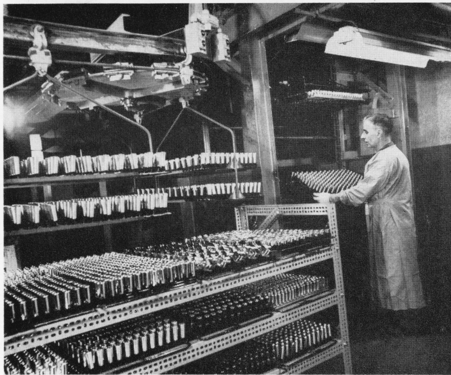
ROUND AND ROUND THEY GO. The gleaming lipstick caps which Domenic Cherasulo is unloading from the baking oven conveyor line will be placed on the "run-around" overhead conveyor and carried into the assembling and packing departments of our newly automated Cosmetic Container Division. The Division occupies two floors of Buildings 109 and 112 on East Main St. in Waterbury.
